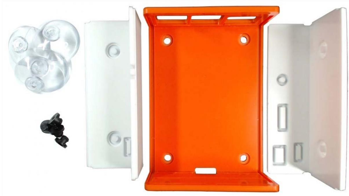
**Step 2** – To install the rubber feet on the bottom part of the case you will either have to push and twist them through one of the 4 the holes or help yourself with a small screwdriver to tuck in the top part of the feet within the hole as shown on the left. Be careful not to cut through the feet and rather than using the tip of the screwdriver use the flat surface to push the head of rubber foot in.
