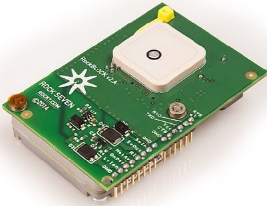
RockBLOCK with built-in patch antenna
